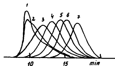
Fig. 1. Experimental chromatograms of dextran standards (numbers as in Table I).
